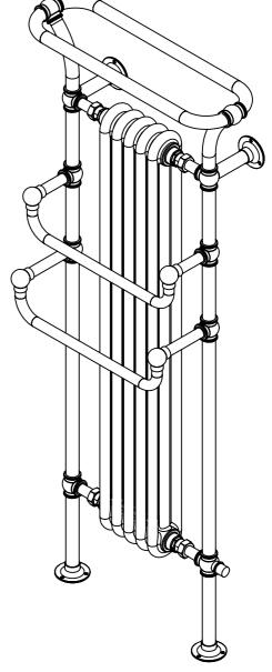
BTU/HR AT DELTA 60: 5328 TEST PRESSURE: 6 BAR ELECTRICAL ELEMENT WATTAGE: 250 MAX WORKING TEMPERATURE: 100°C
